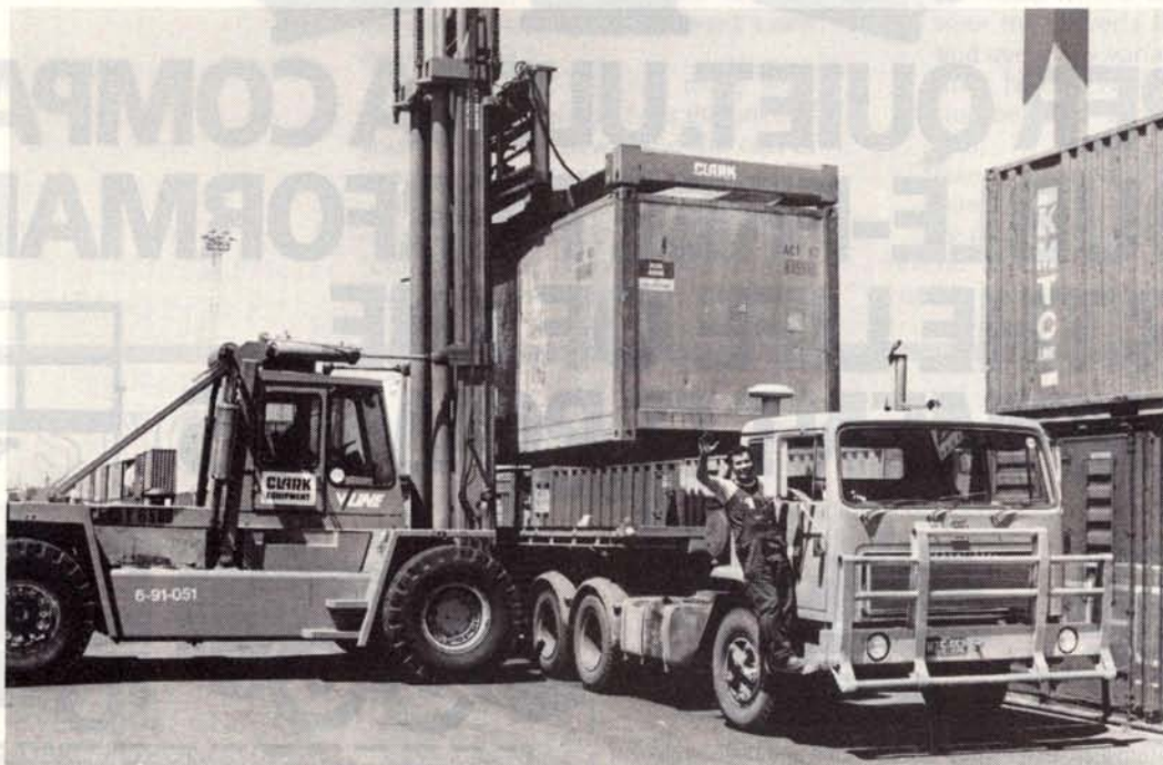
Wreckair Containers being off-loaded from road to rail transport at V/Line's South Dynon Depot in suburban Melbourne.
