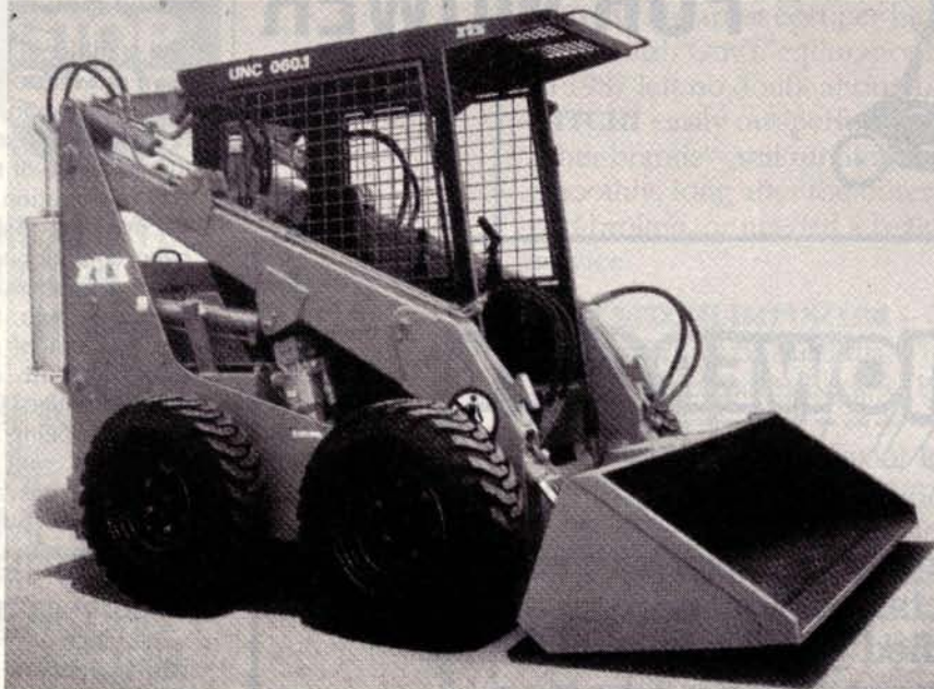
NO CHAINS. The UNC 060 has hydrostatic drive to all four wheels, as well as independent brakes. It also has a ROPS cabin and 15 types of attachments.
